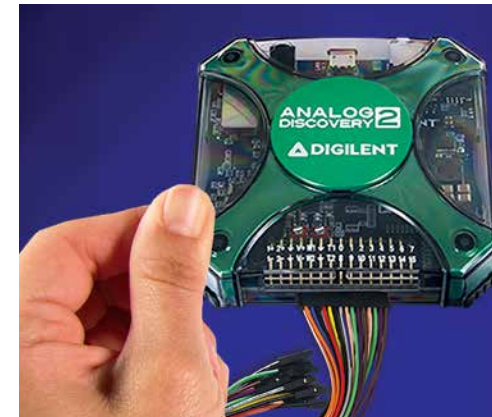
The Analog Discovery 2 kit, manufactured by Digilent Inc. and developed in conjunction with Analog Devices, is a low-cost portable USB oscilloscope, logic analyzer and variable power supply that can replicate the functions of bulky and expensive desktop lab bench test equipment.
