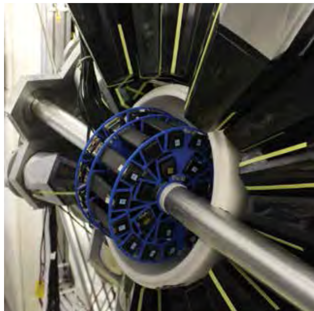
NEUANCE at the center of the DANCE array. A 2 centimeter thick Li-loaded polyethylene shell is installed between NEUANCE and DANCE at Los Alamos Neutron Science Centre, Los Alamos National Laboratory.
