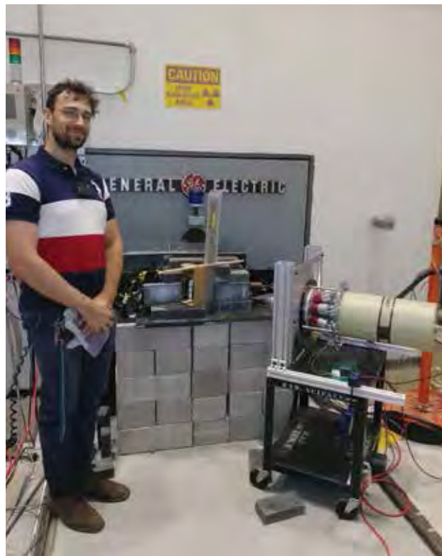
Graduate student Razvan Stanescu works with the multi-detector setup to measure fission gamma rays from U-235 at the thermal column of the UML Research Reactor.
