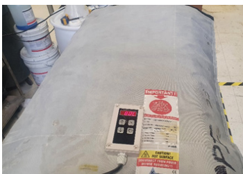
Figure 1. Image of the sandwich panel to be cured under a heat blanket set to 80°C.
